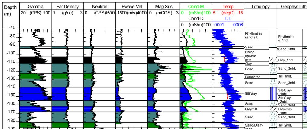
Figure 7: Physical Property Logs for GSC-BH-NOB-01 - Responses to Grain Size Sequences in Lower Sediments
