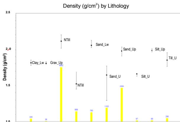
Figure 5: Density Box-and-Whisker Plot based on General Lithologies from 3.5" PVC Cased Boreholes
