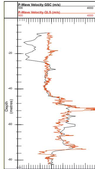
Figure 2: GSC and QLS P-Wave Velocity (m/s) Data for OGS-PJB-15 (Existing data from Pullan, et al., 2000)
