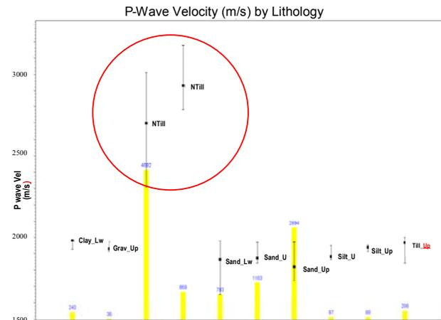
Figure 4: Box-and-Whisker Plot showing P-wave Velocity Contrast between Newmarket Till and other ORM Lithologies
