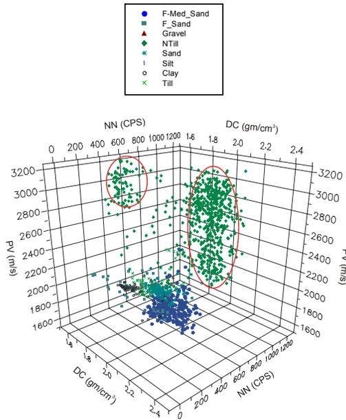
Figure 6: Neutron (NN)/Density (DC)/P-wave Velocity (PV) Multihole 3-D Cross-Plot showing Two Distinct Clusters of Newmarket Till.
