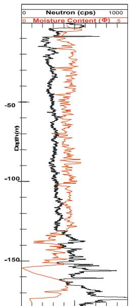
Figure 8: Neutron and Moisture Content Correlation for hole CVC-ORM-01b
