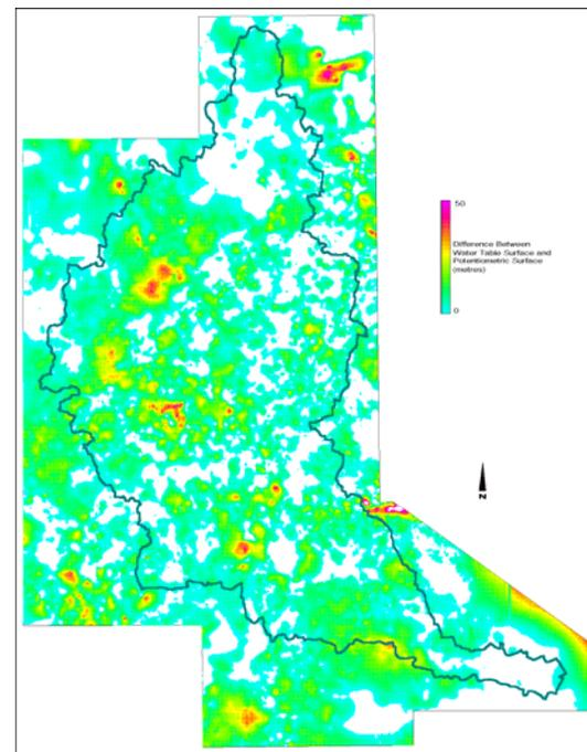
Figure 3. Areas showing downward hydraulic gradients
