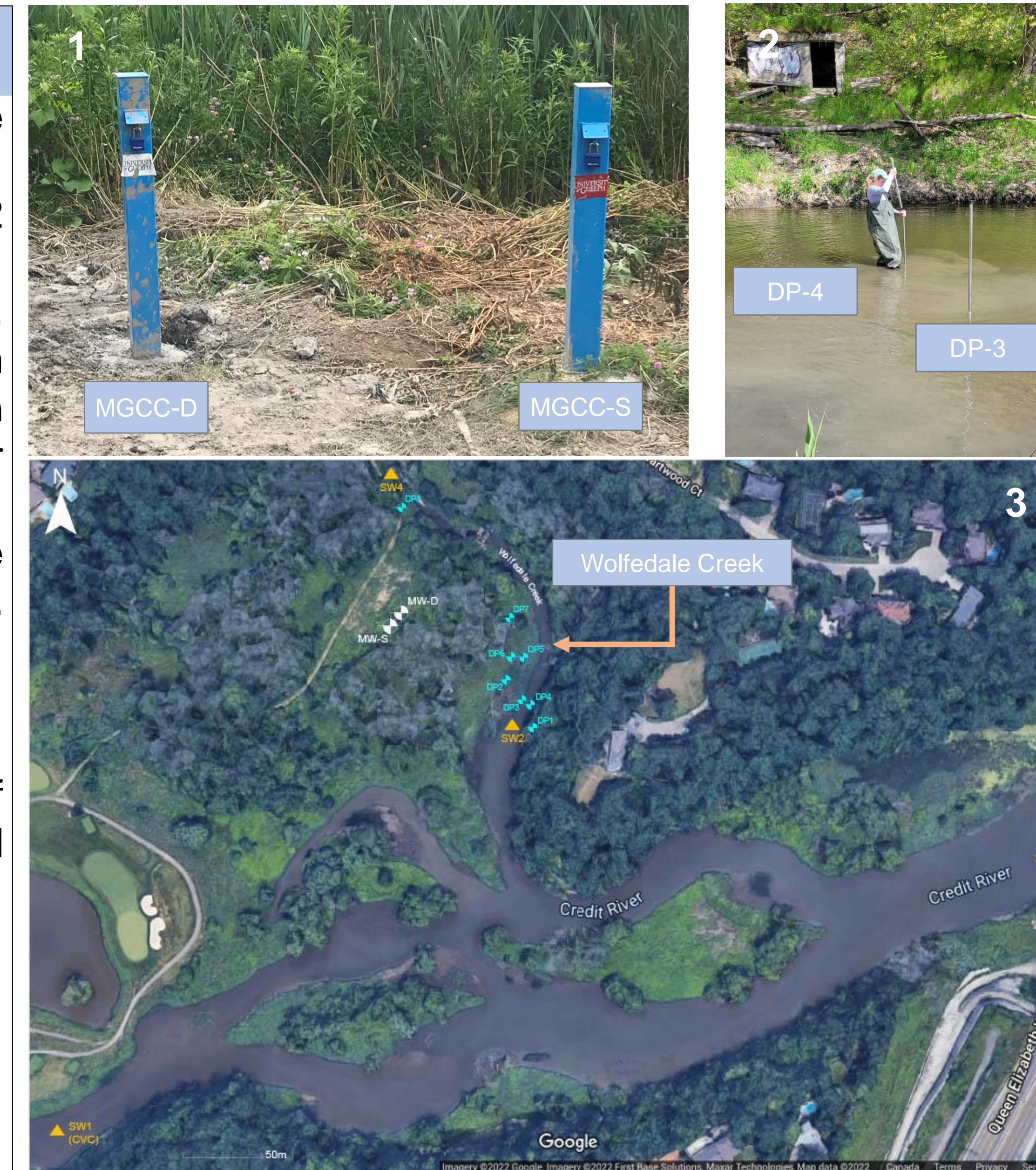
Figure 2. (1) Wells drilled at MGCC, (2) drive point piezometers installed in stream at MGCC, (3) site map of MGCC infrastructure.
